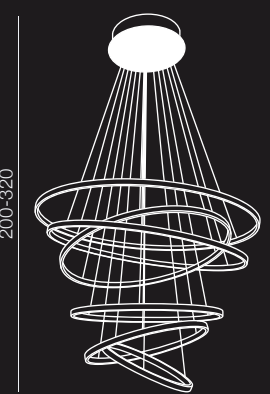
Ø 85 LED Wheel 6 MP57011-6A (chrome) LED 135W 8800 lm chrome/metal
